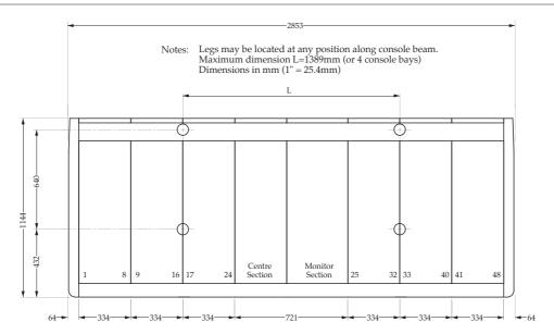
The **C200** console is constructed in bays of 8 channel strips, providing flexible frame options. The position of the centre section may be located at any bay boundary, and a variety of frame options, including producer sections, angles, split points for shipping and installation, and a script tray, may also be specified.
