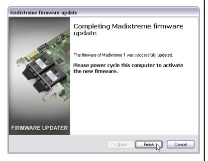
It is most important that power be removed from the computer for a short period after the firmware has been updated. This is because MadiXtreme only loads the new firmware image into the hardware on power-up and if power is not removed your new image will not be loaded...
