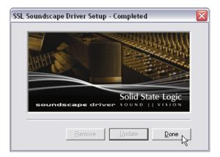
• At the end of the process you will see **SSL Soundscape Driver Setup – Completed** in the title bar. Click **Done**, shut down the computer and move on to installing the hardware.
