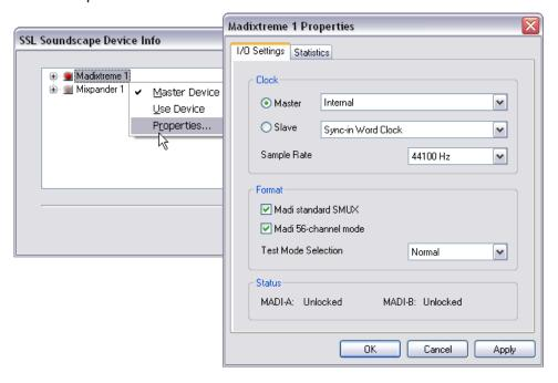
• The MadiXtreme Properties window is divided into three sections. The top section (Clock) allows you to define the clock settings you require for your studio. The middle section (Format) controls the audio configuration. The bottom section (Status) shows whether the MadiXtreme is correctly synchronized to a clock signal and whether the MADI inputs are locked to a valid incoming MADI signal.
