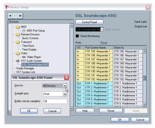
Although the Soundscape drivers allow multiple cards to be used simultaneously, the total number of input or output streams is currently limited to 254 – if the total number of either stream exceeds 254 the audio application will not be able to see or use any of the streams. For instance:
