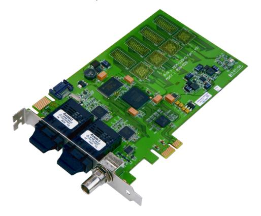
Pull out the protective plugs from the MADI ports on the MadiXtreme and Alpha-Link(s) to gain access to the connectors:
