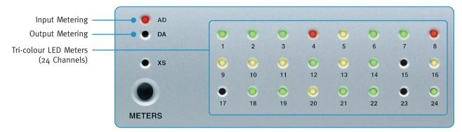
For each input or output channel, the signal level is represented by the state of the LED with the corresponding number. The LEDs respond to the signal level in the digital domain (in dB FS) as follows:
