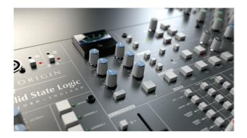
Balanced insert points per channel path (both large and small fader), dedicated channel direct outputs, stem-ready OdB fader bypass switches, plus a new configurable centre section, make ORIGIN an ideal way of adding console workflow to a modern production studio.
