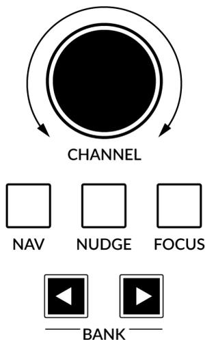
By default, the **CHANNEL** encoder is used to move your DAW tracks across the UF8 surface, in increments of 1 channel at a time. If you find yourself in **NAV** or **FOCUS** modes, simply push the **CHANNEL** encoder to return to **CHANNEL** mode.
