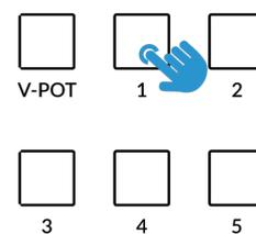
Select User Banks using Keys **1-5** in the **SOFT KEYS** section.
