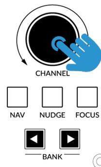
*Press and hold the CHANNEL encoder to enter/exit Transport Mode*
