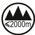
Evaluation of apparatus based on altitude not exceeding 2000 m. There may be some potential safety hazard if the apparatus is operated at altitude exceeding 2000 m.
