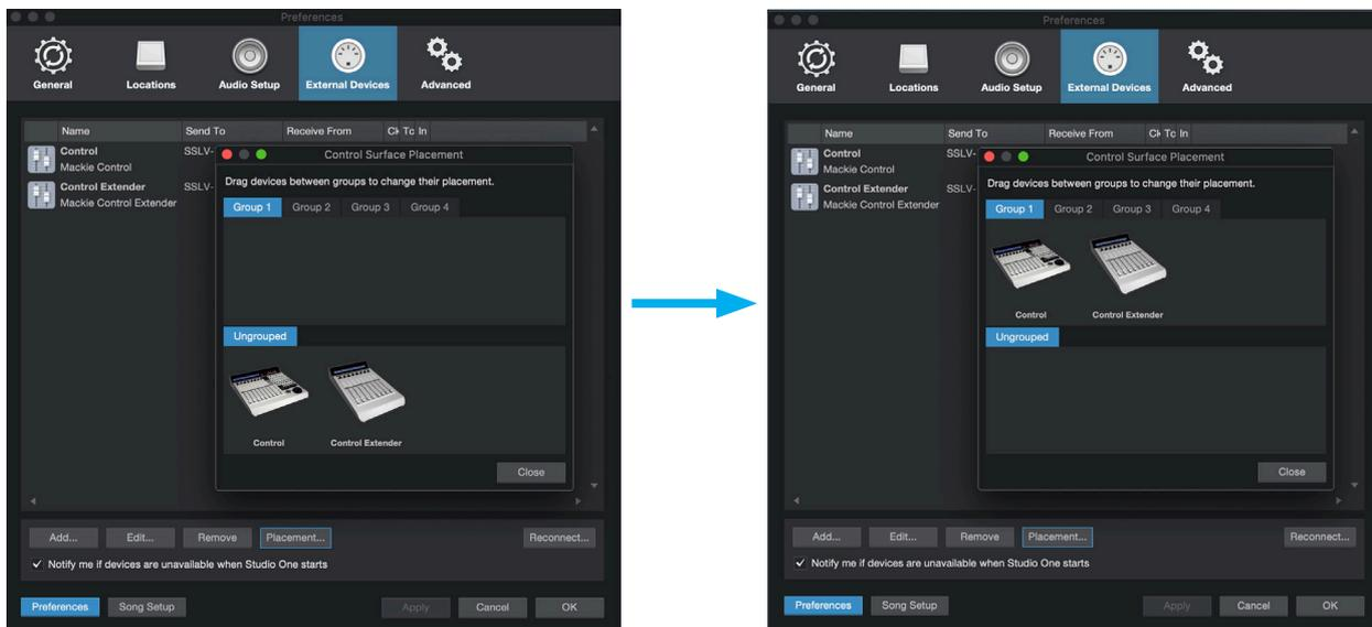
*STEP 7 : Go to Control Surface Placement setup and click and drag the Mackie Control and Mackie Control Extender(s) and move them up into Group 1.*
