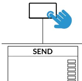
Repeatedly pressing the **SEND** key will cycle the V-Pots through controlling a specific Send 'slot' across all tracks at once. The particular send slot being controlled is reflected by the lighting of the **SEND / PLUGIN** Number Keys 1-8 on the left-hand side.
