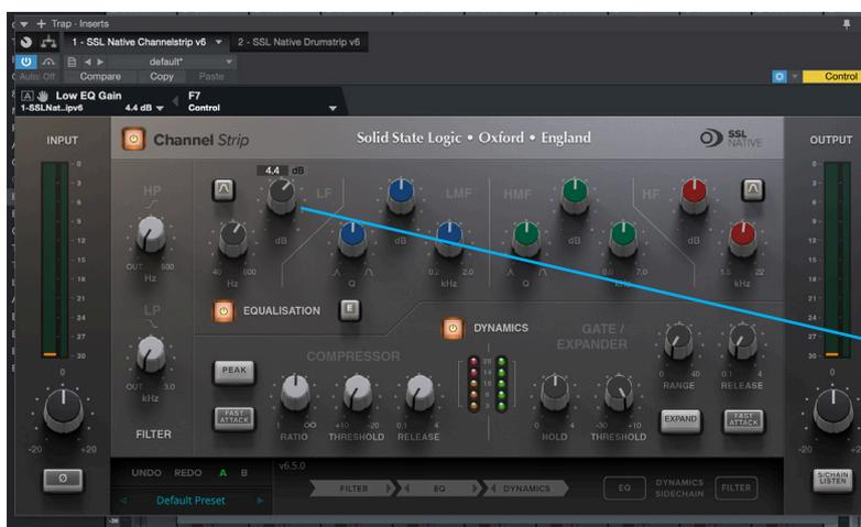
Adjust a parameter - in this example, we're moving the LF Gain control
