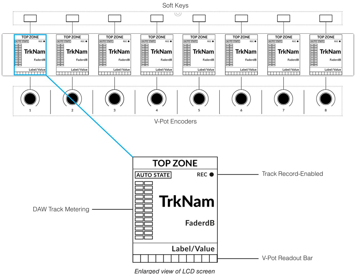
**Top Zone** - Provides a label for the function assigned to the soft key directly above.
