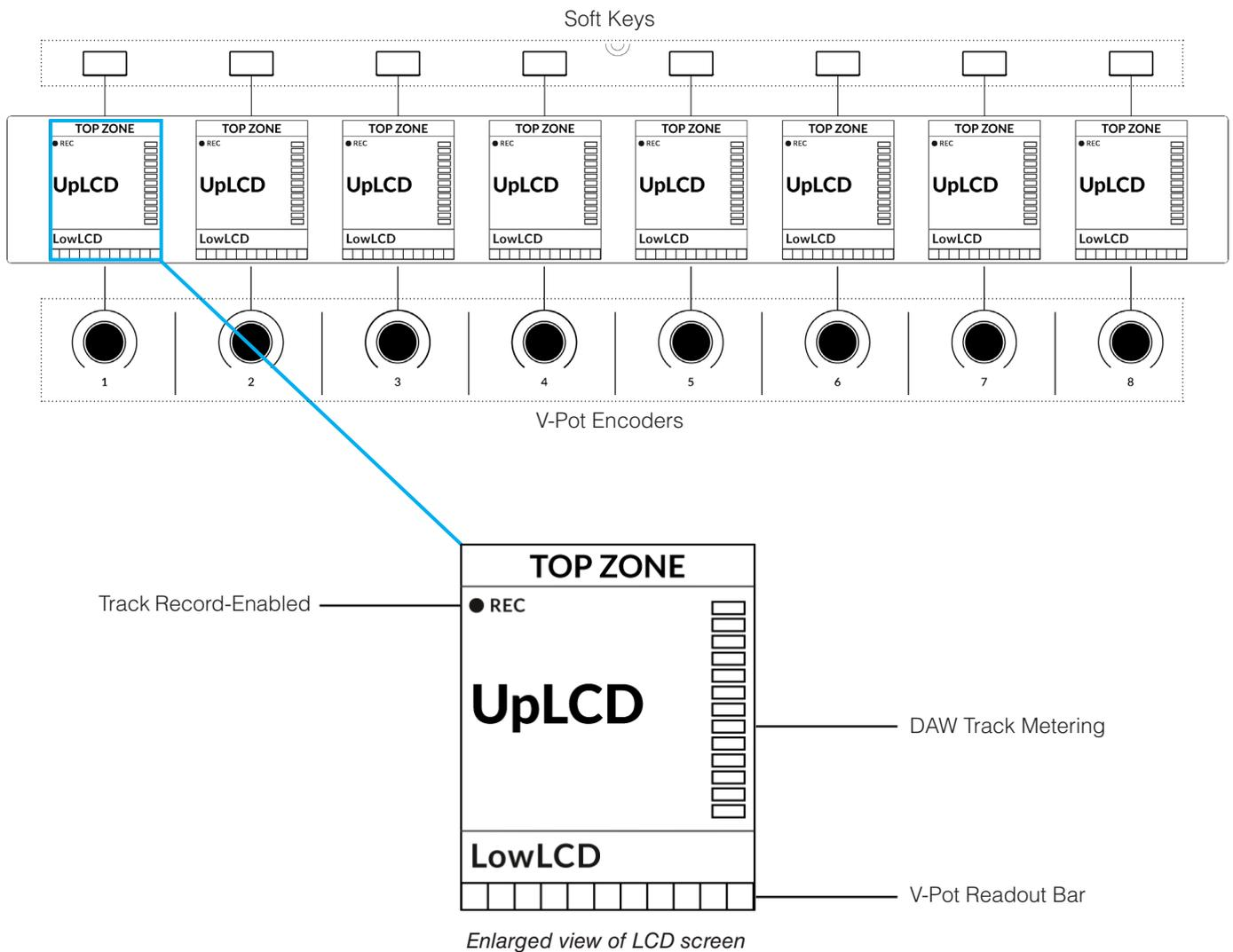
**Top Zone** - Provides a label for the function assigned to the Soft Key button directly above.
