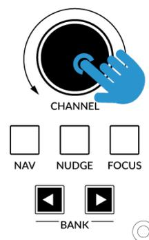
*Press and hold the CHANNEL encoder to enter/exit Transport Mode*
