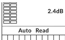
Selected tracks will show their current automation state next to the **Auto** text in the lower section of the LCD. Please note that V-Pots have no functionality when **AUTO** selection mode is active. You must return to **NORM** or **REC**.
