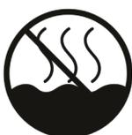
Evaluation of apparatus based on temperate climate conditions only. There may be some potential safety hazard if the apparatus is operated in tropical climate conditions.
