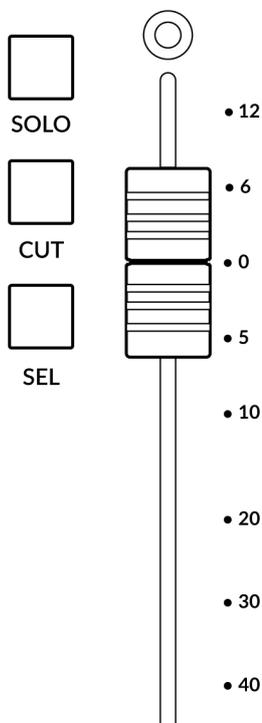
*Touching a single fader will cause the LowLCD area to display a fader dB readout, instead of the V-Pot parameter readout.*
