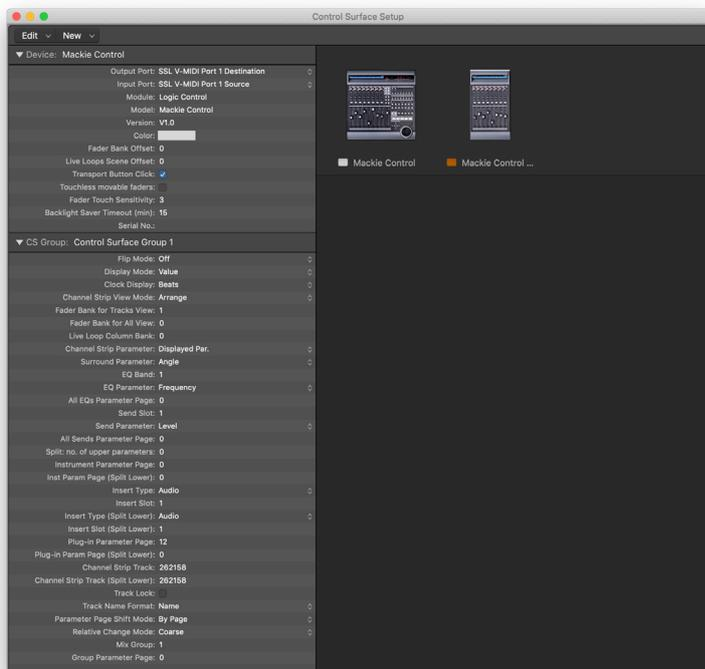
**STEP 8 : Set up the first UF8 as a Mackie Control Unit and subsequent UF8s as Mackie Control Extenders, incrementing the SSL V-MIDI Port number for each Extender.**
