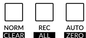
You will notice that there are additional labels beneath the **SELECTION MODE** keys. These functions have no purpose in the Cubase UF8 profile.
