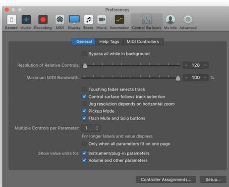
**STEP 5 :** On the 'Control Surfaces' > 'General' tab ensure that 'Multiple Controls per Parameter' is set to '1' and 'Only when all parameters fit on one page' is unticked. Set 'Maximum MIDI Bandwidth' to 100%.
