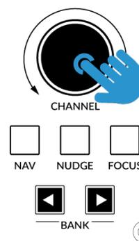
*Press and hold the CHANNEL encoder to enter/exit Transport Mode*
