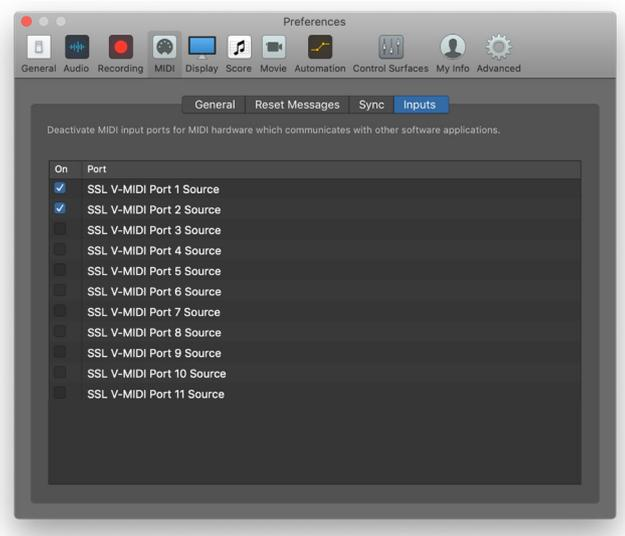
**STEP 7 : Enable SSL V-MIDI Port(s) in Logic.**
