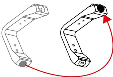
2. Rotate the stands so that the short side fixes to the chassis
