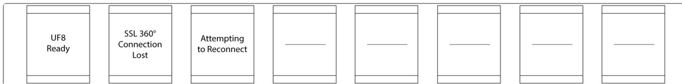
The LCD message above means that communication between SSL 360° and UF8 has been lost. If you experience this, then check that your USB cable connecting UF8 and 360° has not been removed. Re-connect if so.
