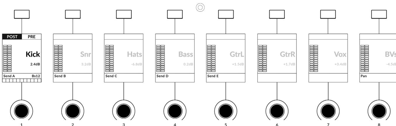
*STEP 3: Use V-Pots 1-5 to control Sends A-E and V-Pot 8 to control Pan.*
