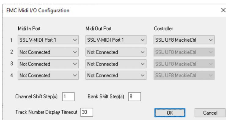
STEPS 8, 9, 10 : Click on the Properties button. Set SSL V-MIDI Port 1 for both Midi In and Midi Out ports. If you have 2 UF8s, set the second port (second UF8) to SSL V-MIDI Port 2 input and output. In the Controller drop-down menu, select SSL UF8 MackieCtrl. Press OK to close the different windows.
