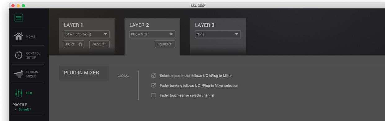
**Selected parameter follows UC1/Plug-in Mixer** - With this mode enabled, the channel strip or Bus Compressor parameter assigned across the V-Pots will automatically change in response to the parameter being moved/actioned in the Plug-in Mixer, on UC1 or in the plug-in itself. e.g. if you move the LMF Frequency control in any of these places, UF8's V-Pots will automatically switch to control that parameter.
