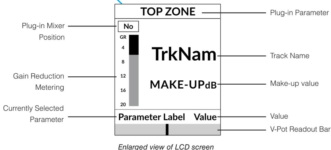
**Top Zone** - Provides a label for the function assigned to the Soft Key button directly above. In the case of the Plug-in Mixer, these Soft Keys are used to select the Bus Compressor plug-in parameter that gets assigned to the V-Pots.
