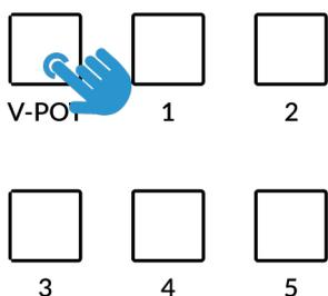
STEP 1 : Press V-POT a second time to toggle Soft Keys keys into Send Mute Mode.
