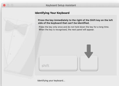
STEP 4: When presented with the message 'Press the key immediately to the right of the Shift Key', press and hold the 360° key on UF8 for 3 seconds until it lights orange.
