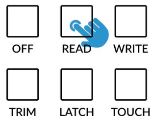
*Set the automation mode for whole mixer using the AUTOMATION keys.*
