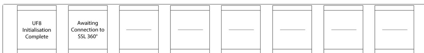
'UF8 Initialisation Complete' means that the UF8 hardware boot sequence has completed. 'Awaiting Connection to SSL 360°' means that UF8 is waiting for the SSL 360° software to start running on the computer. You may see this message appear when logging onto your computer, before the operating system has finished loading your user-profile and start-up items. You may also see this message if you are yet to plug a USB cable from your UF8 into your computer.
