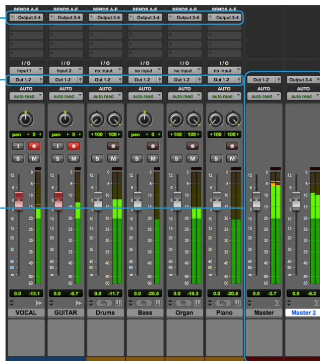
Example of Pro Tools | First Mixer Window Set Up For 2 Different Headphone Mixes
