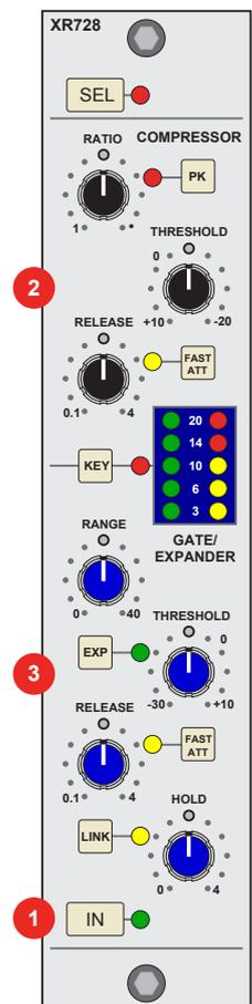
**FST ATT** – Normally, a controlled linear attack time of 1.5ms per 40dB is provided. Press this button to select a fast attack time (100µs per 40dB). The attack time is the time taken for the Gate/Expander to ‘recover’ once the signal level is above the threshold. When gating signals with a steep rising edge, such as drums, a slow attack may effectively mask the initial ‘THWACK’, so you should be aware of this when selecting the appropriate attack time.
