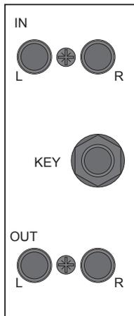
The module inputs and outputs are balanced, connecting via ¼" stereo jack sockets. A single Key input is provided, also connected via a ¼" stereo jack socket. The module is configured to operate at a nominal level of +4dBu; operation at a nominal –10dBV level is not possible with this module.
